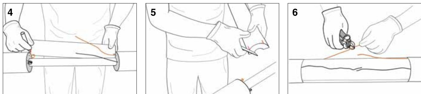
Measure for the PUR insulation shell and cut to the correct length. Make sure there are no gaps between the insulation shell and insulation of the pipe.
