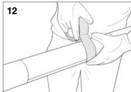
Fasten the PUR insulation shell with duct tape.
