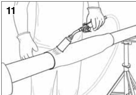
Slowly heat up the end of the PE shrink casing with even and light movements all the way around until the PE shrink casing has reduced to the casing pipe. Be sure the flame is moving constantly to prevent overheating.
